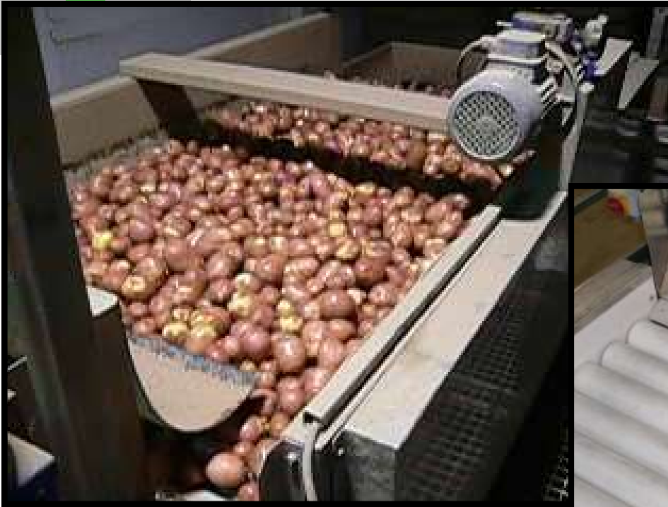
Potato dryer for productions of 5 to 25 Tn/h.
