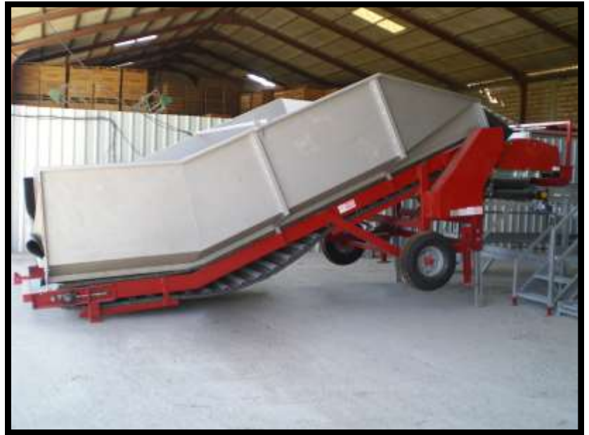
Mobile infeed hopper Mod.2000. Production of 25 Tn/h.
