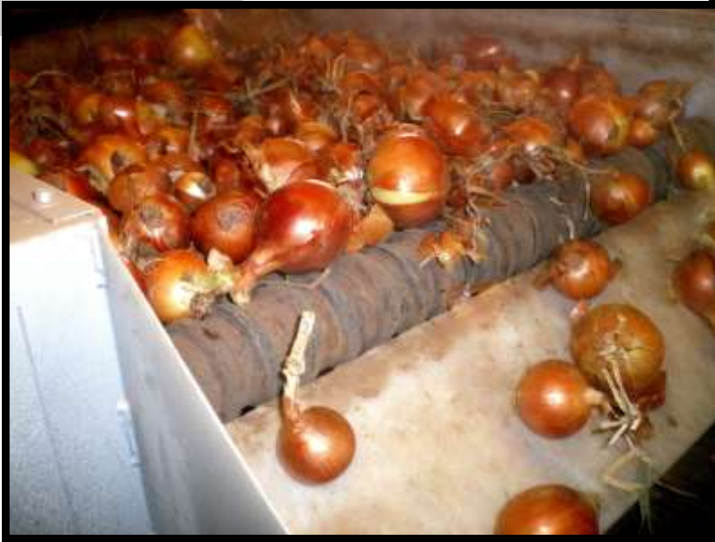
Clod and leaves remover with helical gums working with onions.
