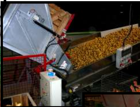
Model for boxes with lower platform to remove empty boxes and lung-type conveyor belt for product reception. Assembly to increase the number of boxes unloaded per hour.
