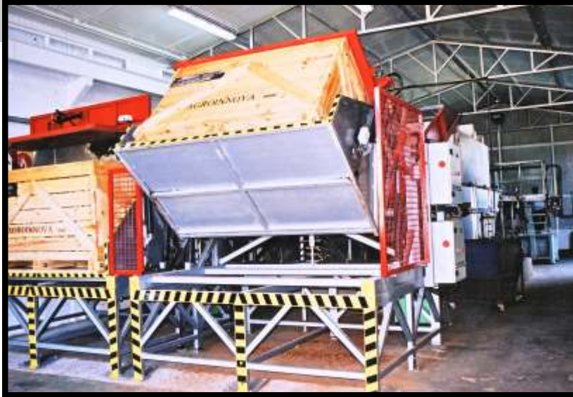
Heavy duty box tipper with automatic hydraulically operated clamp lid and flow door.
