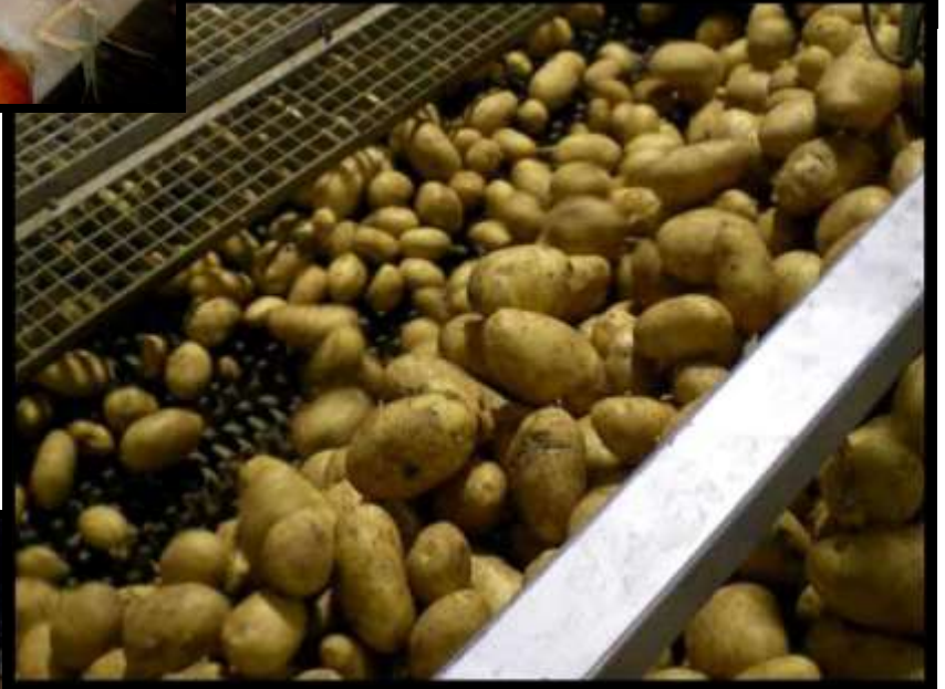
Detail of the clod separator finishes. Inlet, outlet and sides are made of PVC to avoid friction of the product with the chassis
