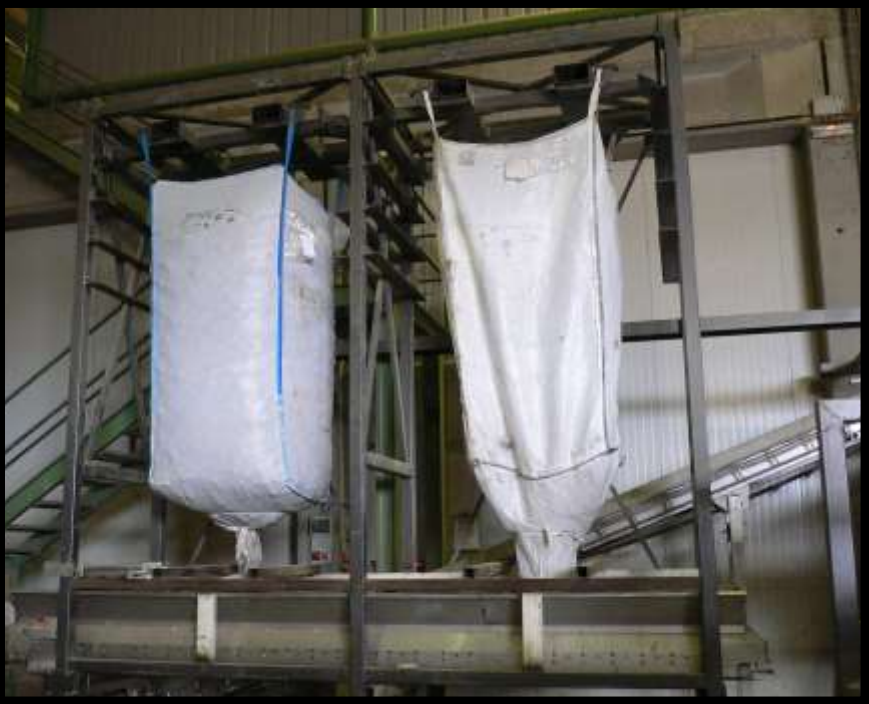
Shelf for two big bags with a lower conveyor belt
