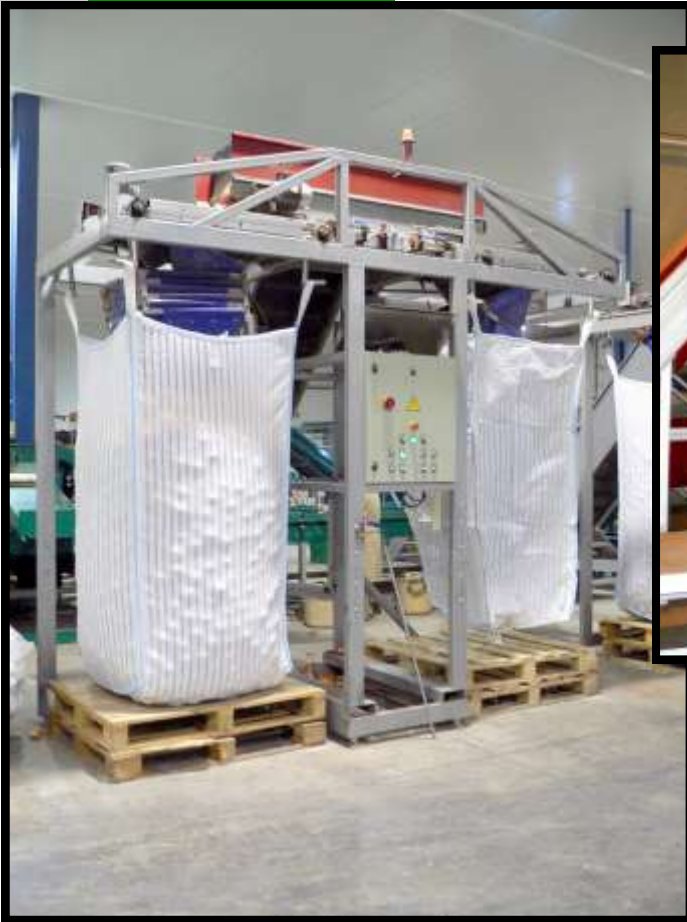
Powered cascade model, ideal for productions of 10Tn/h with a very gentle handling of the product, as it discharges at low height.
