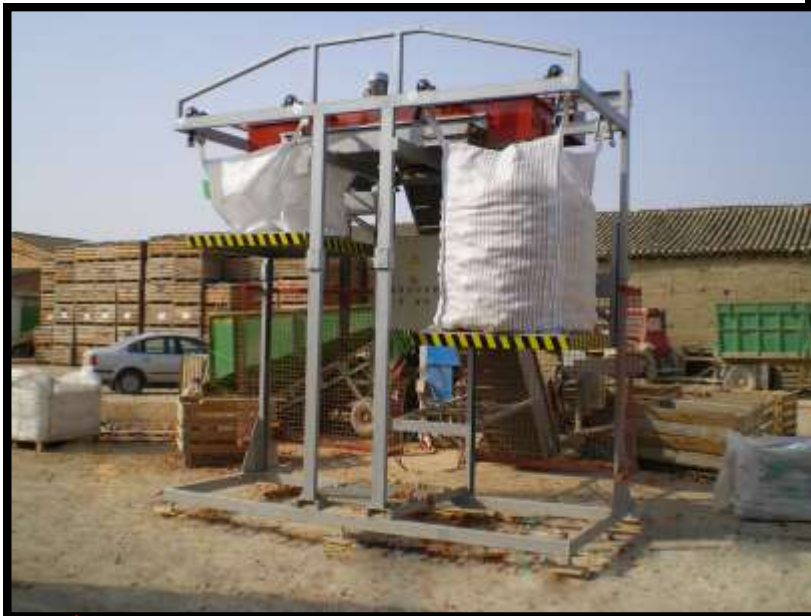
Electromechanical model for productions of 25 Tn/h. The process is completely mechanical, very quiet and with a very reduced initial height of discharge, achieving a very gentle handling of the product.
