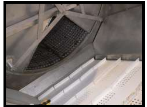
Drum built with perforated sheet flared for the good treatment of the product.
