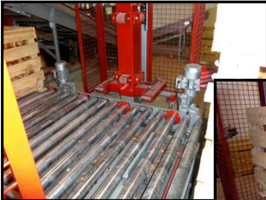
Detail of the system of lifting boxes and of the system of roller conveyors.
