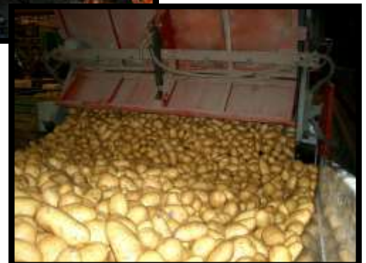
Big Bag tipper set with lung-type receiving conveyor and screen grader.
