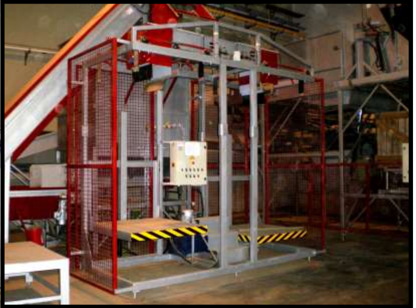
Hydraulic model for productions of 25 Tn/h. Very robust machine with a gentle handling of the product. As in all models, the uncoupling of the bag is automatic.
