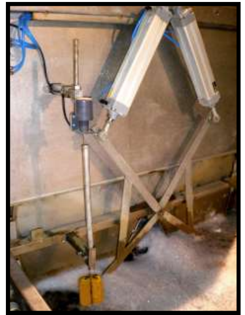
Pneumatic opening system for the doors of the submerged drum washing machine
