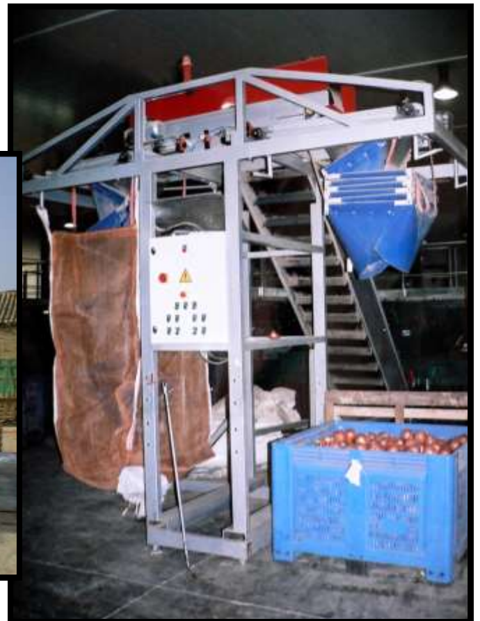
Powered cascade model that is unloading simultaneously into a bag and a box.
