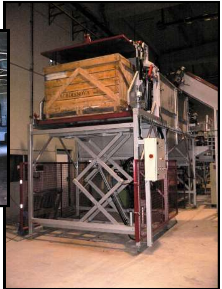
Model for boxes with lower platform to remove empty boxes and lung-type conveyor belt for product reception. Assembly to increase the number of boxes unloaded per hour.
