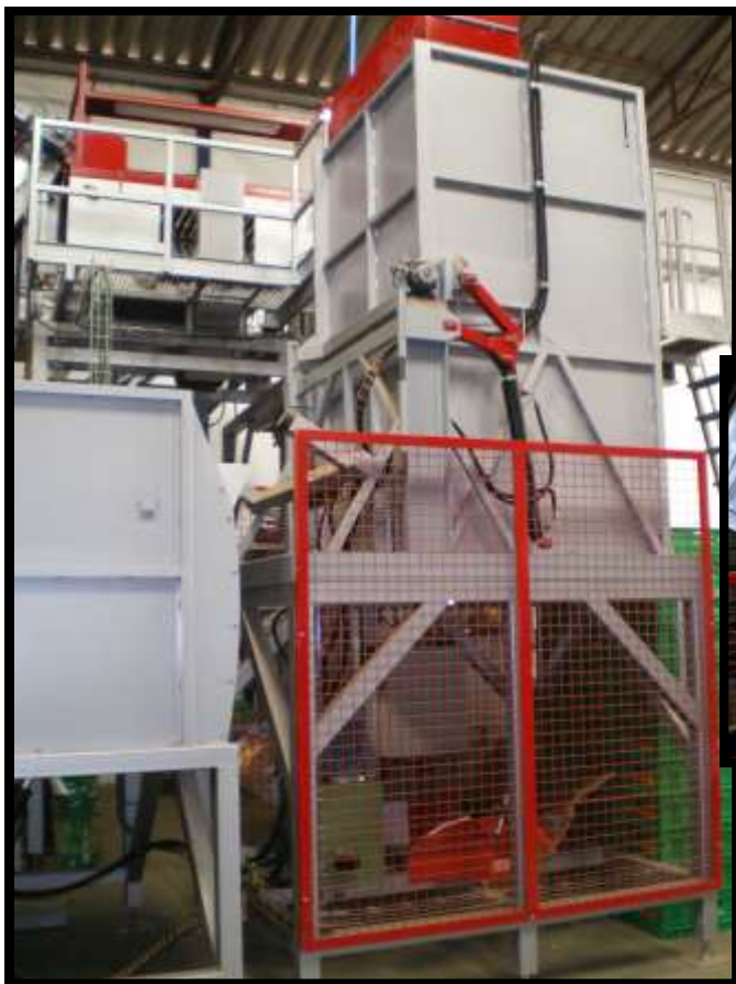
Big Bag tipper with manually adjustable fixed clamp lid and automatically flow door.
