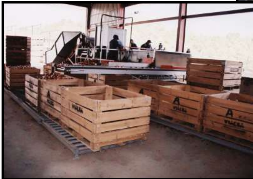
Detail of the roller path. It increases the speed and ease of unloading.
