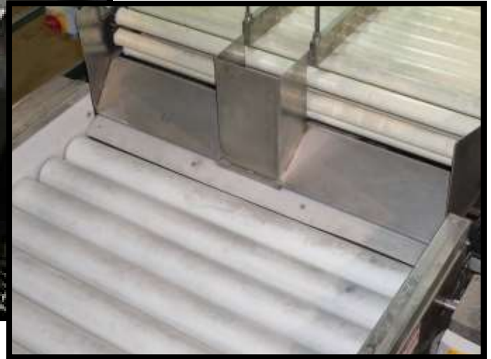
Detail of the potatoes dryer. The sides are made of PVC for the best handling and treatment of the potatoes.
