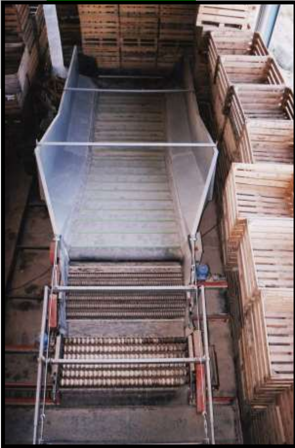
Maxihopper set for increased product capacity with pre-grading screen at the output
