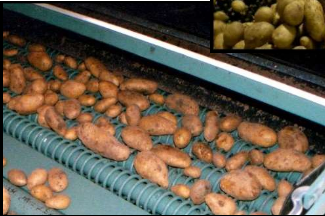
Spring separator model working with potatoes. The production of these machines is from 5 to 25Tn/h depending on the width and number of rollers. All models have a gentle touch of the product. The width of the machine is designed according to customer needs, as well as the loading and unloading height of the product
