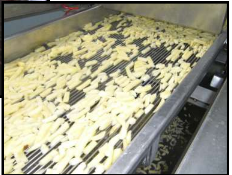
Blanching machine with "jacuzzi" system to improve the distribution of the antioxidant throughout the surface of the sliced potato.
